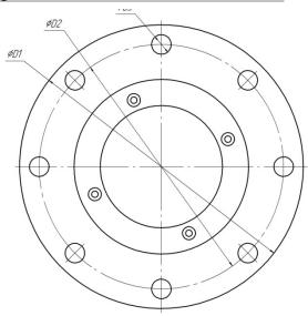
Depending on the order, the ULM level transmitters can be completed with various installation (adapter) flanges as per different standards (GOST, DIN, ANSI, etc.). Request them when placing an order.
